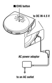
The CD player charges the batteries. The "CHG" indicator turns on in the display, and the indicator sections of [27] light up in succession. When the batteries are completely charged, the "CHG" and [27] indicators turn off.
